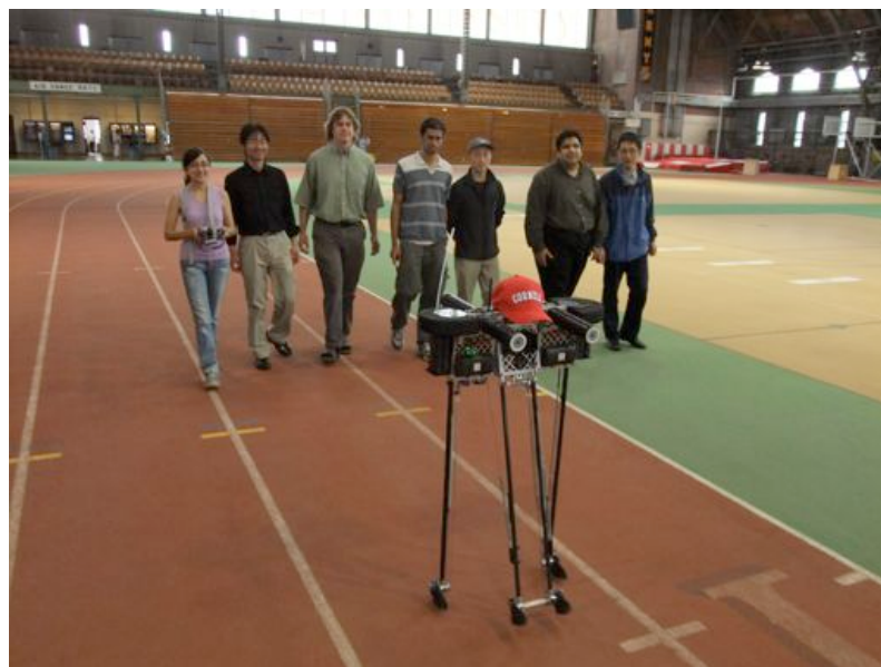
Figure 7.4: Ranger’s ultra-marathon walk. On 1-2 May 2011 [12], Ranger walked non-stop for 40.5 miles (65 km) on Cornell’s Barton Hall track without recharging or being touched by a human. Some of the crew that worked on Ranger are shown walking behind Ranger during the 65 km walk. Basic data are in the table below.
