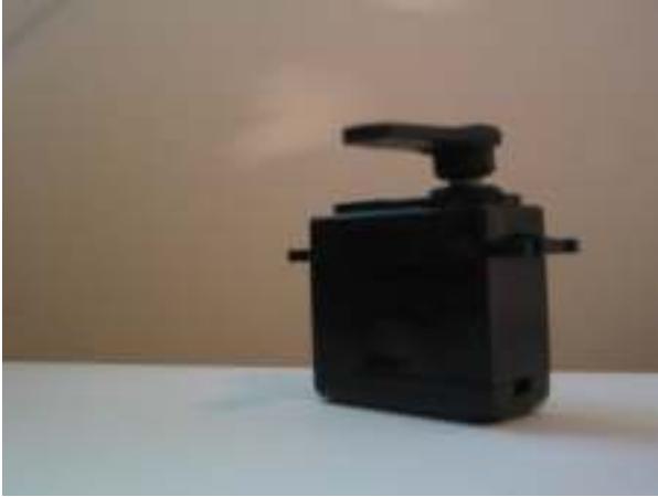
Figure 7: Servo motor used in the steering system.
