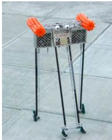
Figure 1. The Cornell Ranger walking robot. It has four legs split into two groups, inner and outer. Each step is made by striking the ground with the foot and then rolling forward into the next step.
