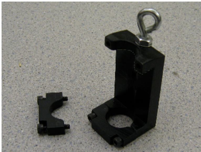
Figure 10: The inner leg bracket as machined
