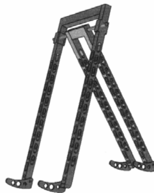
Figure 1: 2-Dimensional Bipodal Walker
