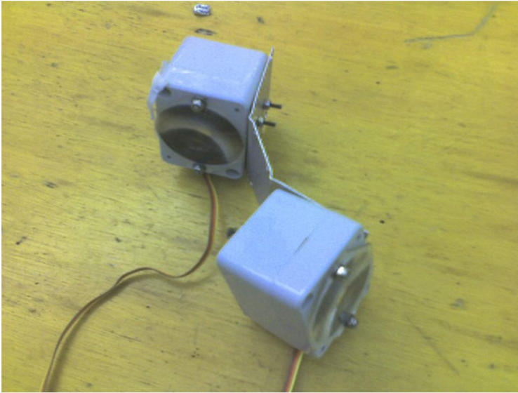
Figure 1. The physical casing of the Avago color sensor.
