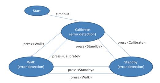
The graph shows that switching of states is controlled by input of UI button. The first state after starting up is Calibrate state.
