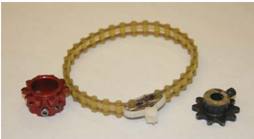
Failed Sprockets and Chain
