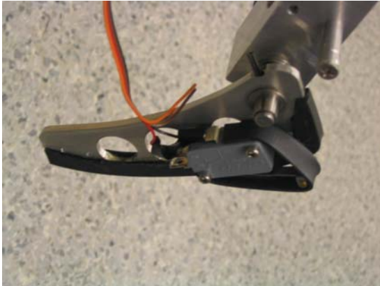
Figure 14 – Single limit switch replaces dual limit switch system. A rubber sleeve was placed over the steel lever of the switch to protect it from damage.
