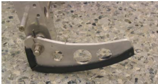
Figure 13 – Rubber U-channel sole installed on foot
