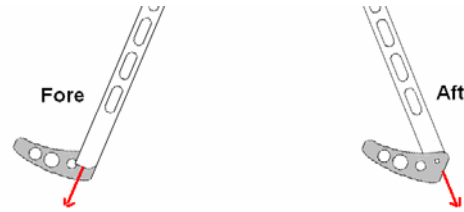
Figure 14 – Components of force directed along the walker legs that present problems when walker is in a static stance.
