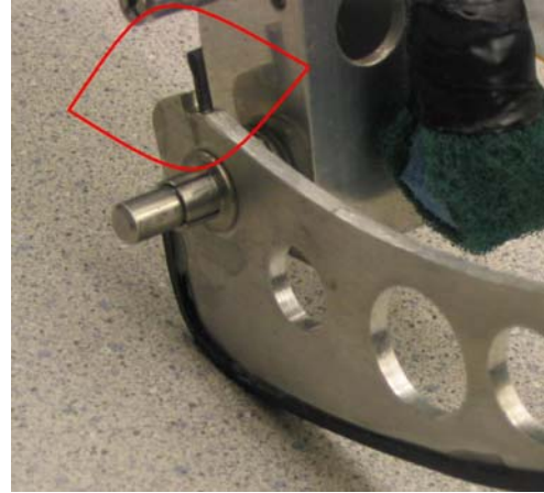
Figure 11 – Circled area shows spring pin inserted through the top of a foot into an ankle shaft
