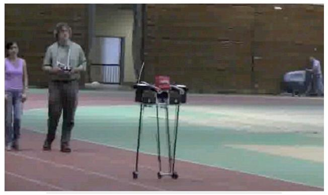
Marathon: Cornell University's Ranger robot broke the world record for continuously walking without needing to be recharged or even touched by engineers
