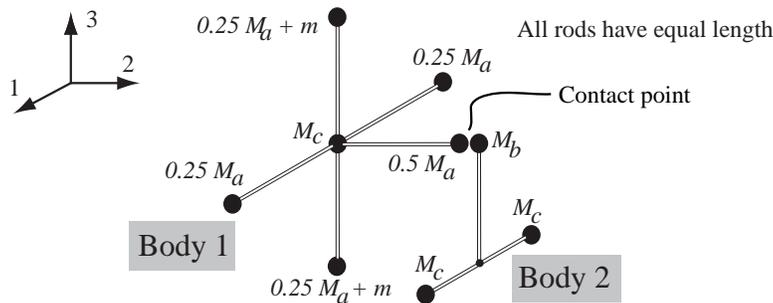
FIGURE 0.2. Physical realization of arbitrary mass matrices
