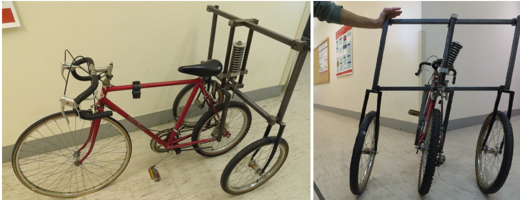
Figure 1. A ‘bricycle’: a vehicle which can transition between bicycle and a tricycle. It is a bicycle with two extra ‘training’ wheels at the back on a spring-loaded parallelogram mechanism. The spring resists bicycle lean, more or less depending on its adjustment. When the spring is removed the training wheels are mechanically invisible, effectively reducing the bricycle to a bicycle. When the spring is locked the bicycle is effectively a tricycle. The neutral point in-between is the main topic of study here.
