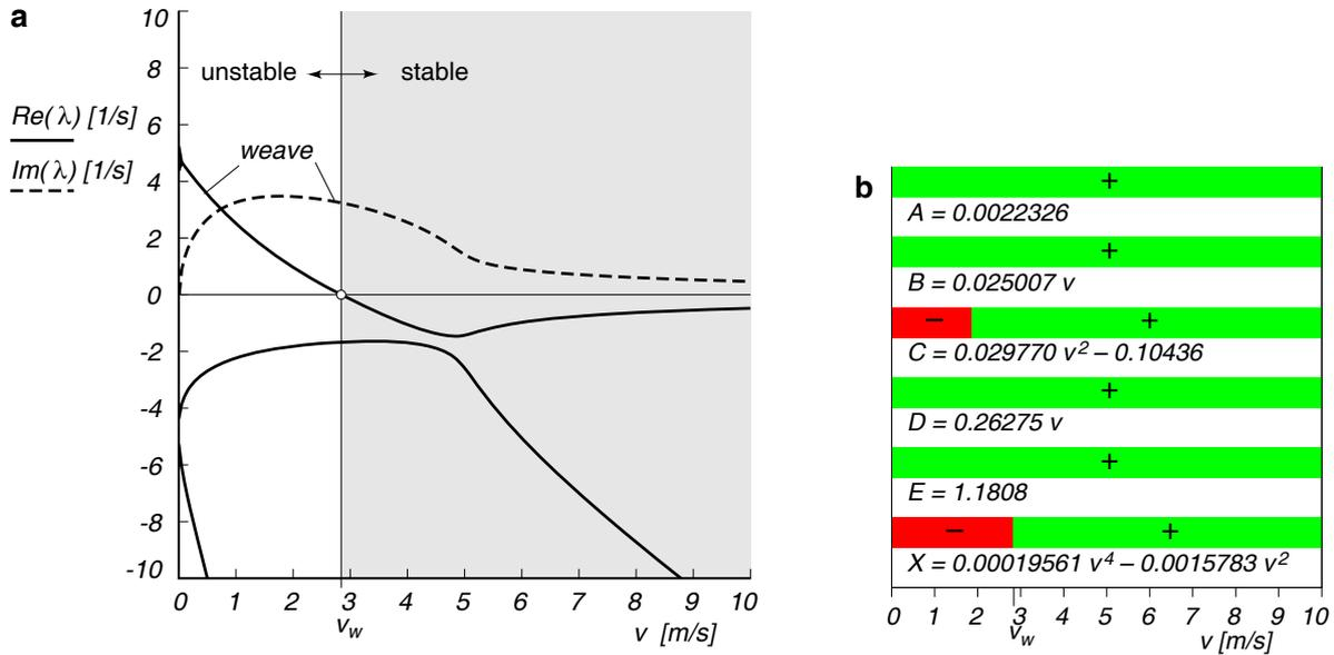
Figure 7.2: **a)** Eigenvalues and **b)** Characteristic polynomial coefficients  $A \cdots X$ . The bars show the speeds where the coefficients are positive (green) for a theoretical two-mass-skate (TMS) bicycle from Figure 7.1 and Table 7.1 in a forward speed range of  $0 \leq v \leq 10$  m/s. Note that the real parts of all eigenvalues are negative for  $v > 2.8$  m/s.
