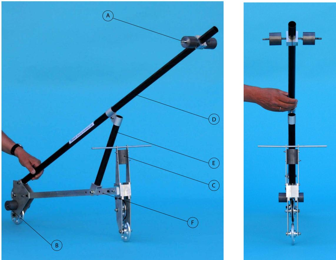
Figure 9.1: **left**) Overview of the experimental two-mass-skate bicycle, with (A) 2 kg rear frame forward point mass, (B) 2 kg point mass at the rear contact point, (C) Point mass front frame, (D) Rear frame upper tube, (E) Rear frame support tube (F) Lower rear frame member. **right**) Front view of the experimental two-mass-skate bicycle.
