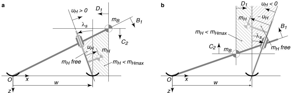
Figure 7.3: **a)** Allowed location for the front mass  $m_H$  (shaded areas) for which the two-point-mass bicycle to be stable when  $\lambda_s > 0$ ; **b)** the same but now when  $\lambda_s < 0$ . The shaded regions are described in the text.
