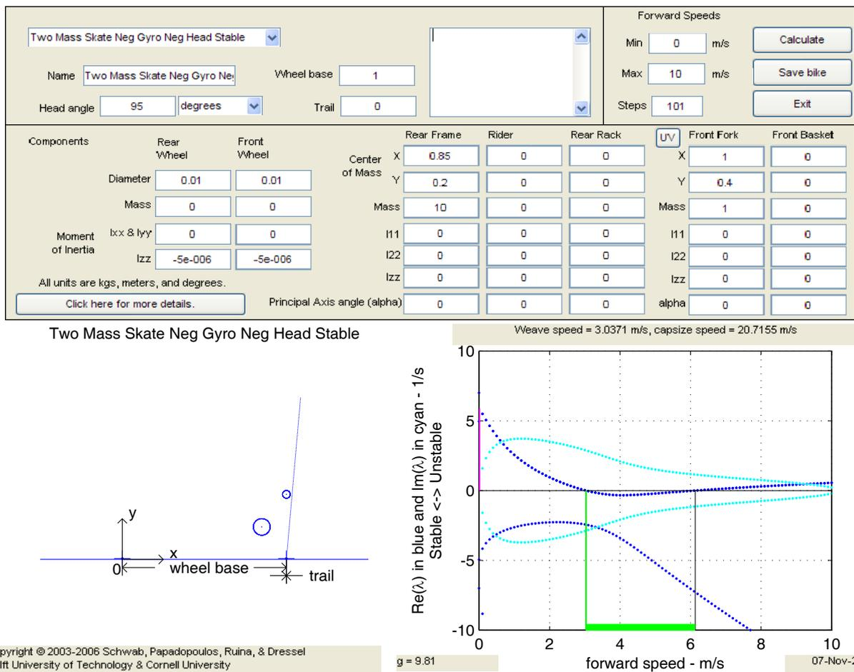
Figure 6.7: A two-mass-skate (TMS) bicycle with negative gyroscopic action, reverse tilted steer axis, which shows a stable forward speed range. The model is based on the alternative theoretical two-mass-skate (TMS) model from Chapter 7, which has a reverse tilted steer axis with added negative gyroscopic action. This bicycle clearly shows a stable forward speed range.
