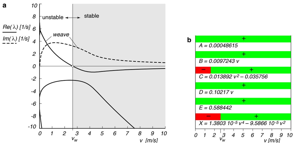
Figure 7.5: **a)** Eigenvalues and **b)** Characteristic polynomial coefficients  $A \cdots X$  (green when positive) for the *alternative* theoretical two-mass-skate (TMS) bicycle from Figure 7.4b and Table 7.2 in a forward speed range of  $0 \leq v \leq 10$  m/s. Note that for  $v > 2.6$  m/s the real parts of all eigenvalues are negative.
