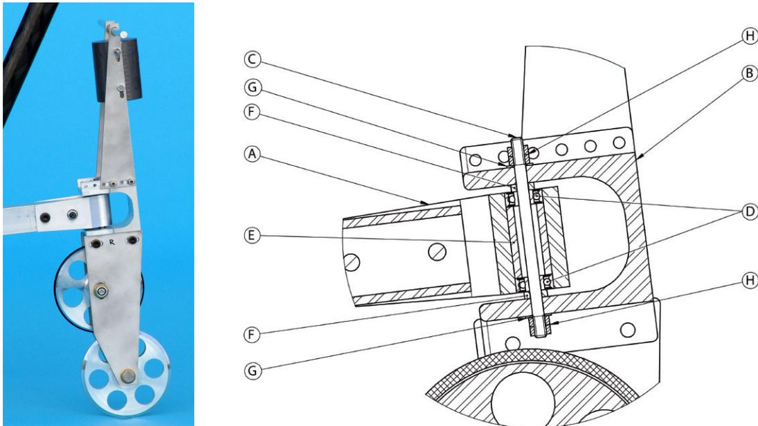
Figure 9.2: **left)** Side view of the front assembly of the experimental TMS bicycle. **right)** Front frame and steering head cross-section. (A) Rear frame head bracket, (B) Front frame head bracket, (C) Dowel with threaded ends, (D) Bearings, (E) Glued bearing spacer, (F) Spacer, (G) Washer, (H) Nuts.
