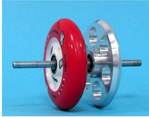
Figure 9.3: Two different types of 100 mm diameter wheels used, **left:** a polyurethane “inline skate” wheel, which didn’t work, and **right:** the sharp aluminum wheel, with a crown radius of 2 mm, that was used in the experiments presented.
