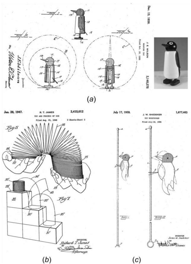
Fig. 1 U.S. Patent drawings of passive dynamic toys. (a) The passive dynamic ramp toy known as the Wilson Walkie, as well as a photograph of the toy. (b) The Slinky, another passive dynamic toy capable of walking down stairs. (c) A woodpecker toy that descends a pole using in a piecewise pecking motion.
