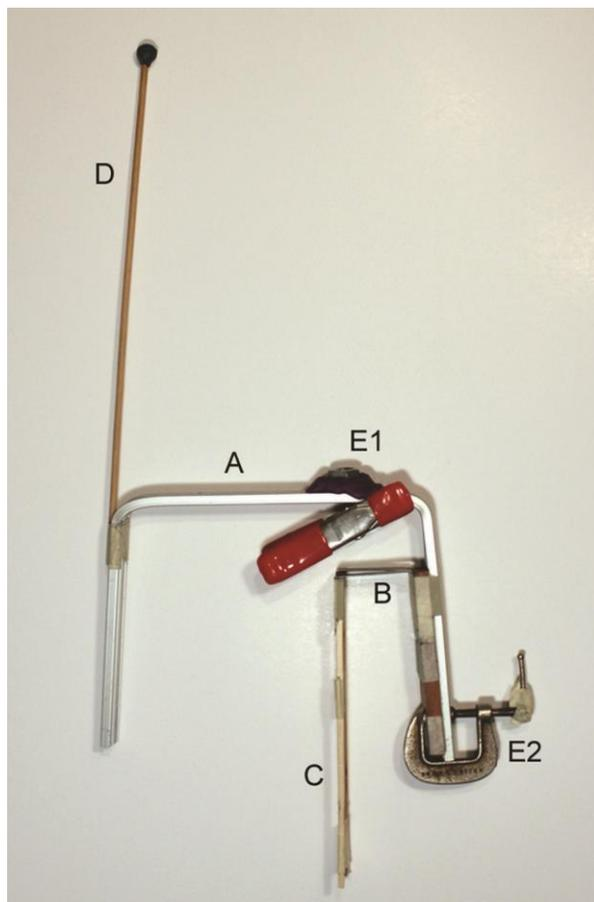
Fig. 5 Early use of leaf spring in hopper. The body frame A was a U shaped bent aluminum extrusion. Leaf spring pair B connected dual wooden legs (chopsticks) C to the frame. The tail mast D was a wooden dowel with clay adhered at top. Clamps and clay were used as adjustable masses E1–E2 (multimedia extension 5 video).
