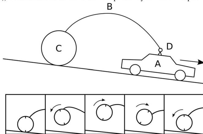
Fig. 2 Ball and car toy. A toy car A is attached by a curved wire spring B to highly elastic rubber ball C. One end of the wire spring is embedded in the ball. The opposing end of the wire spring is attached by hinge D to the top of the toy car. The lower panel shows the approximate orientation of ball during one hop cycle, as the car leads the ball down the hill. Arrows indicate the alternating direction of ball pitching between collisions (multimedia extension 2 video).
