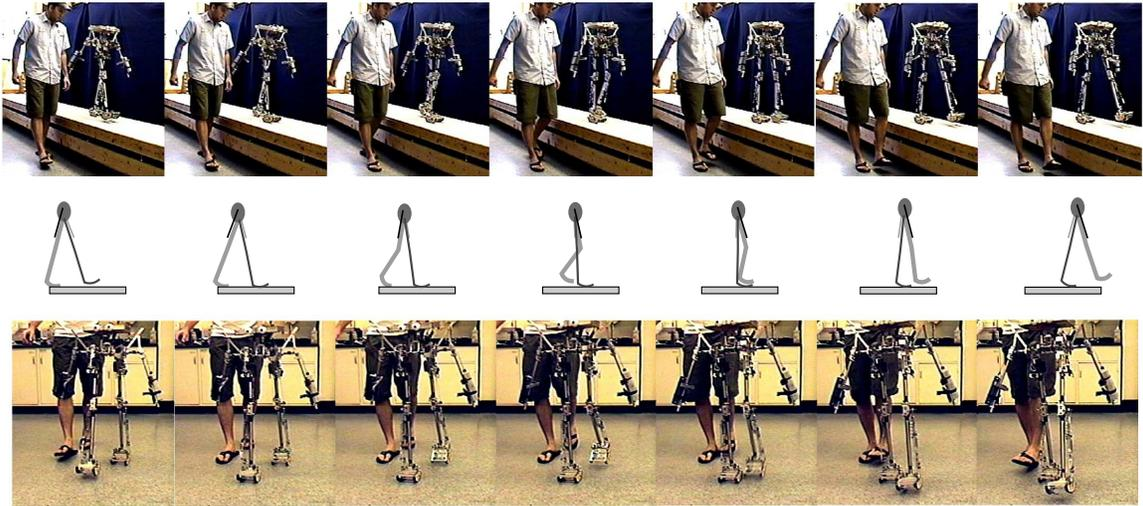
Figure 4: Two sets of video stills of the Cornell ankle-powered biped walking on a level surface next to a person. A little less than one step is shown at 7.5 frames/s. Both the robot and the person are walking at about 1 step/s. The stick figure indicates the leg angles for the corresponding video stills; the right arm and leg are darker than the left.
