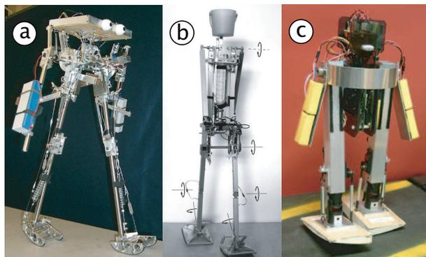
Figure 2: Three level-ground powered walking robots based on the ramp-walking designs of Fig. 1. (a) The Cornell biped. (b) The Delft biped. (c) The MIT learning biped. These powered robots have motions close to their ramp-walking counterparts as seen in the supplementary movies. Information on their construction is in the supplementary text.
