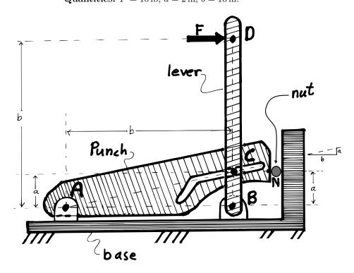
a) (25 pts) Find the force acting on the nut at N. A number is desired (i.e., so many lb force). [Hint: Only substitute in numbers when you have a formula for your answer in terms of a, b and F.]
