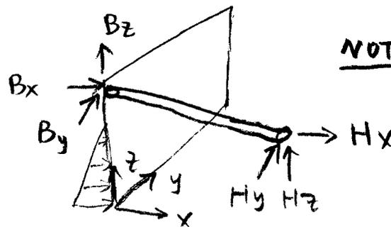
(b) To figure out the axial force in rod BH, we could do moment balance about axis AD. In this way, reactions from the hinge
