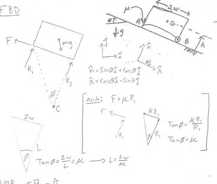
$\frac{\Delta MB_{c}}{F_{G/c}} \sum \vec{M}_{c} = \hat{\vec{H}}_{/c}$   $\vec{F}_{G/c} \times (-mg\hat{S}) = \vec{F}_{G/c} \times (ma\hat{S})$   $\vec{F}_{G/c} = (\frac{2w}{m} + h) \hat{S}_{+} + (-w) \hat{S}_{-}$
