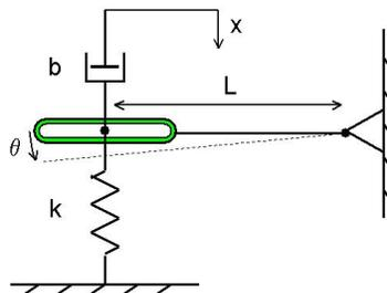
You are given the machine shown above. The input is  $x$ , the output is  $\theta$ . For small  $\theta$  and negligible masses, find the transfer function (assume zero initial conditions). Based on the transfer function, what mathematical operator does this system represent? What type of function is its operand in the time-domain? Find the response if  $x$  is a unit-step.
