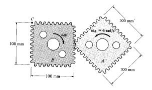
2. Gear A is in mesh with gear B as shown. If A starts from rest and has a constant angular acceleration of  $\alpha_A = 2rad/s^2$ , determine the time needed for B to attain an angular velocity of  $\omega_B = 50rad/s$ .
