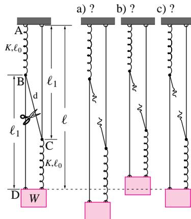
When rope BC is cut does the weight go (a) down?, (b) up?, or (c) stay put?
