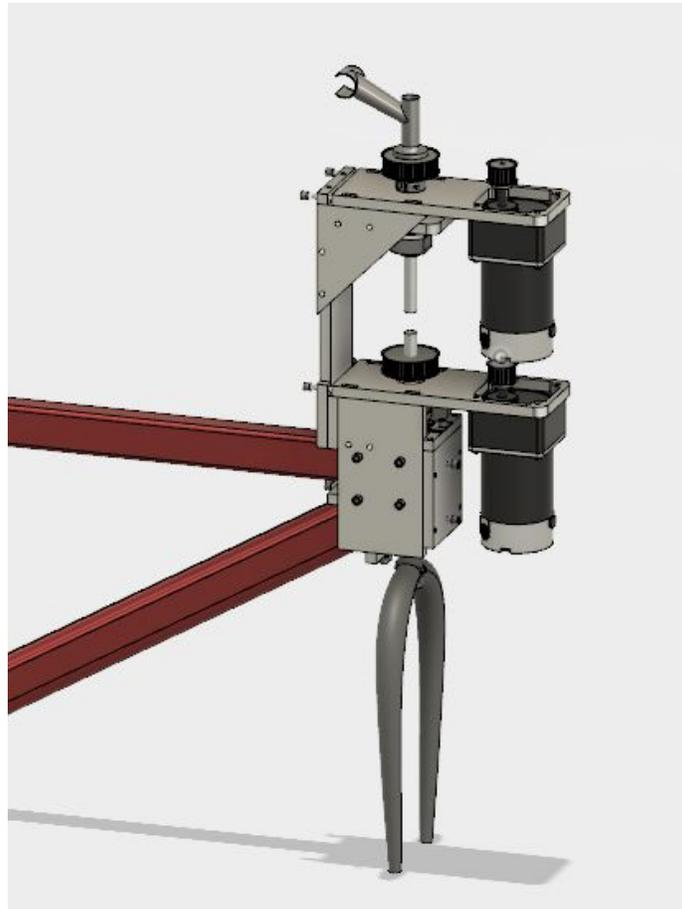
Figure 4: CAD of bike's assembly with motor and power transmission to handlebar
