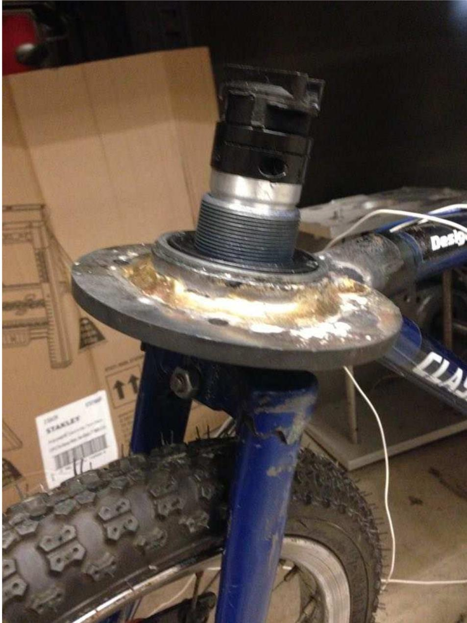
Figure 6.2: front wheel with fork insert and coupling
