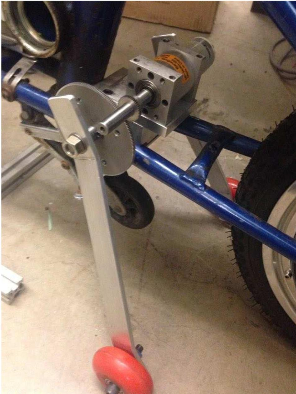
Figure 6.7: wheels, gear and motor connected to bike
