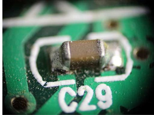
Figure 7.4: Surface-mount capacitor.<sup>4</sup>
