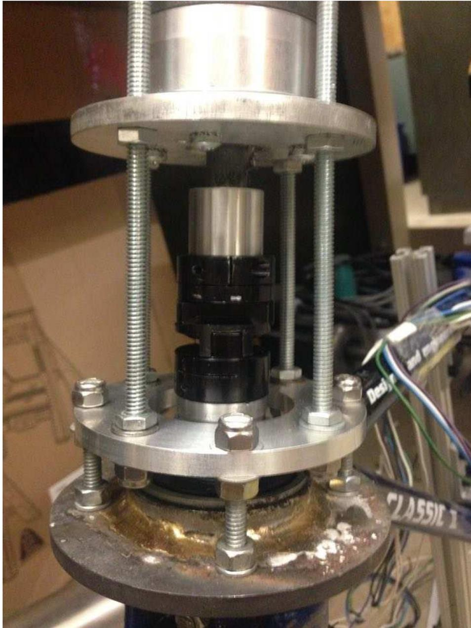
Figure 6.3: plate connected to steel on the bottom and holding the 4 long rods
