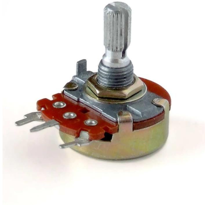
Figure 4.6: An example of a potentiometer. One outer pin connects to the power, the other outer pin connects to ground, and the middle pin is output signal. <sup>6</sup>
