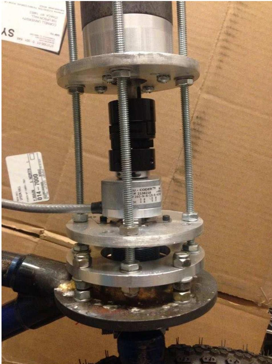
Figure 6.4: the coupling between the motor (top) and the encoder (bottom)
