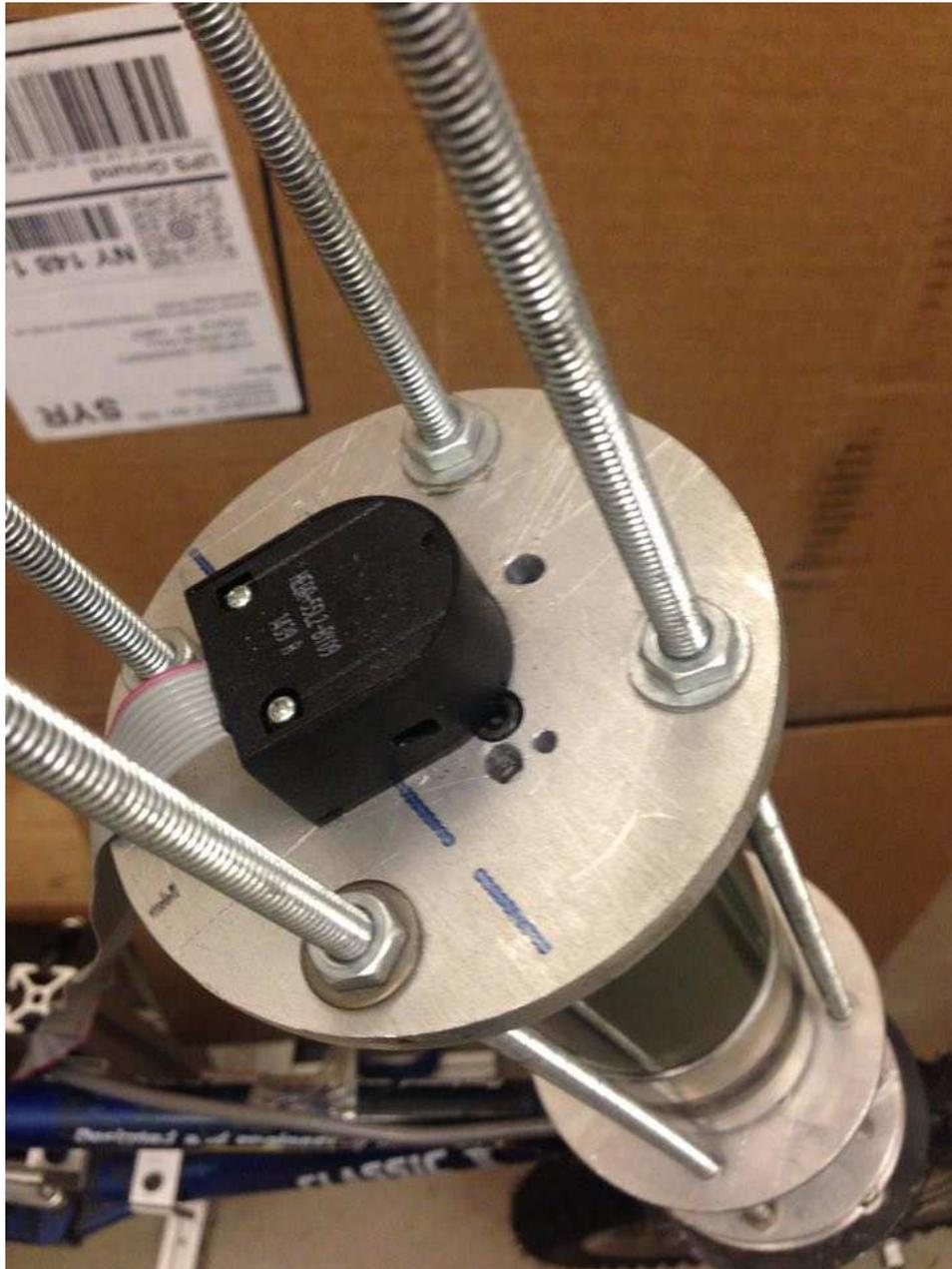
Figure 6.5: the encoder (black box) sits on the end of the motor
