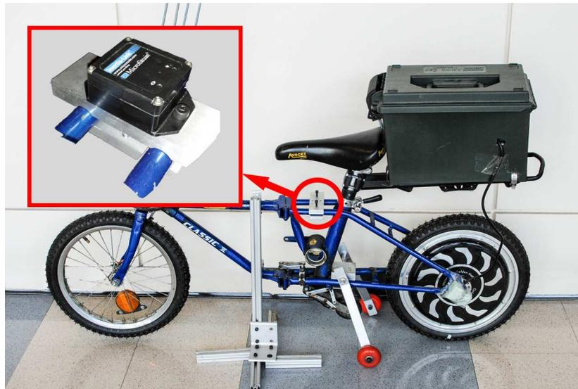
Figure 6.6: the IMU mount is clamped to the bike frame (blue)
