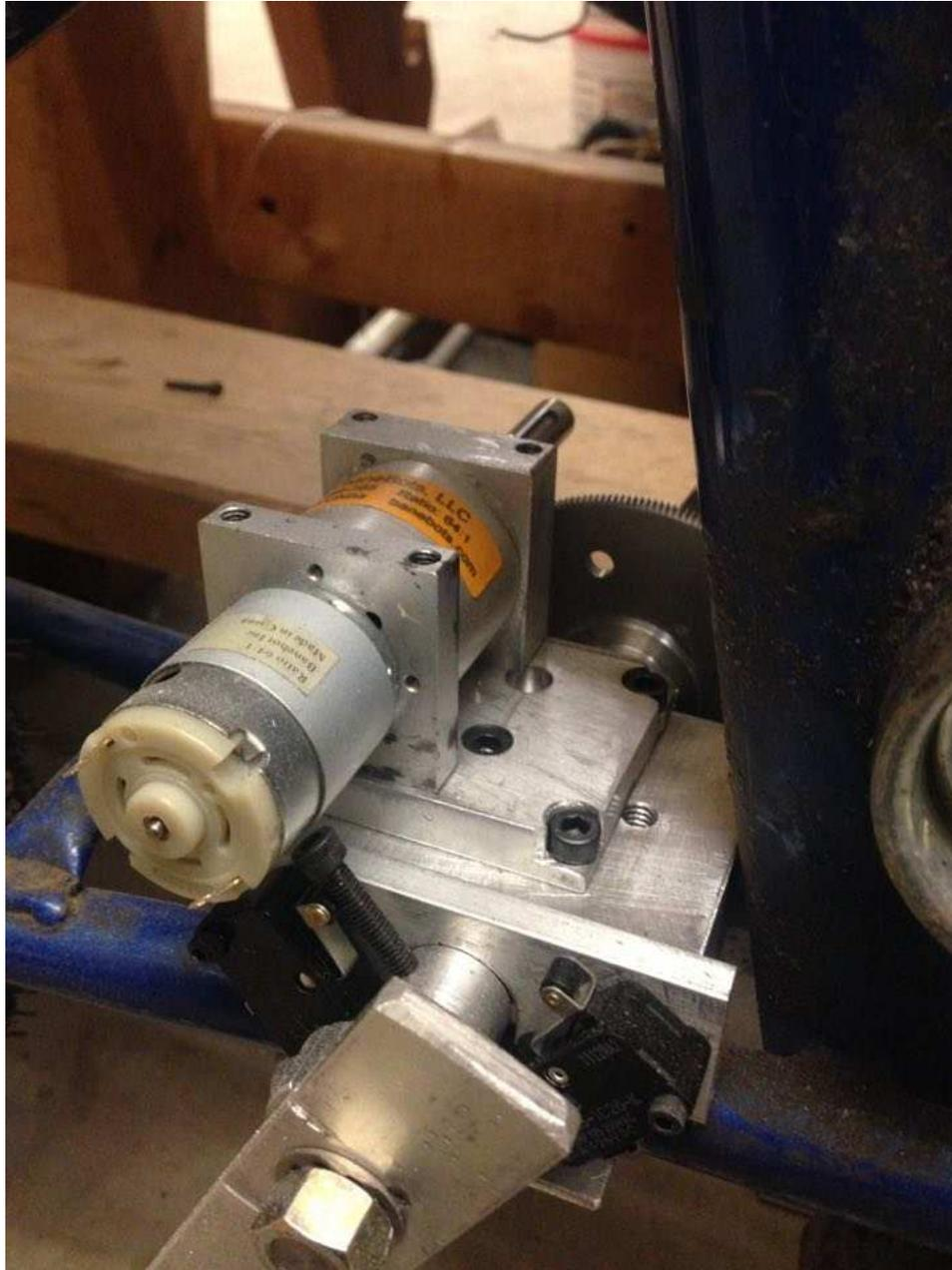
Figure 6.8: reverse side with end-stops
