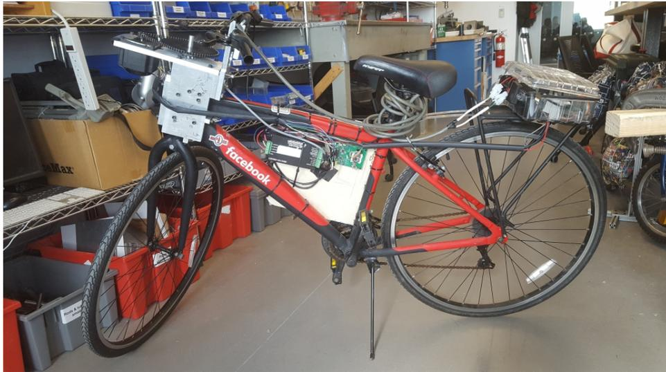
Figure 4.8: Components mounted in front triangle of bike frame. Note the components are not wider than the frame itself, so they do not interfere with the legs on someone riding the bicycle.
