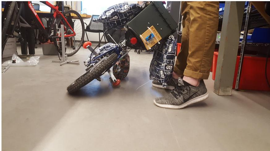
Figure 11.4: Landing Gear Hits Ground before Airbags
