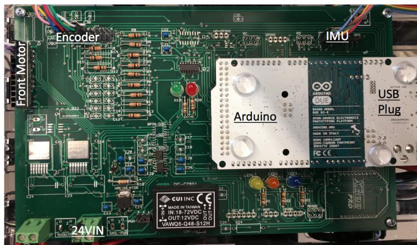
Figure 5.2: This image shows the PCB created for the Steer by Wire Bicycle Prototype. (Note the blank board was purchased from PCB works, and then circuit components were soldered onto the board.)
