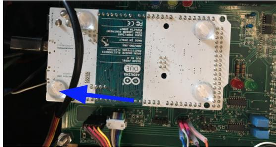
Figure 17.5: Arduino Reset Button
