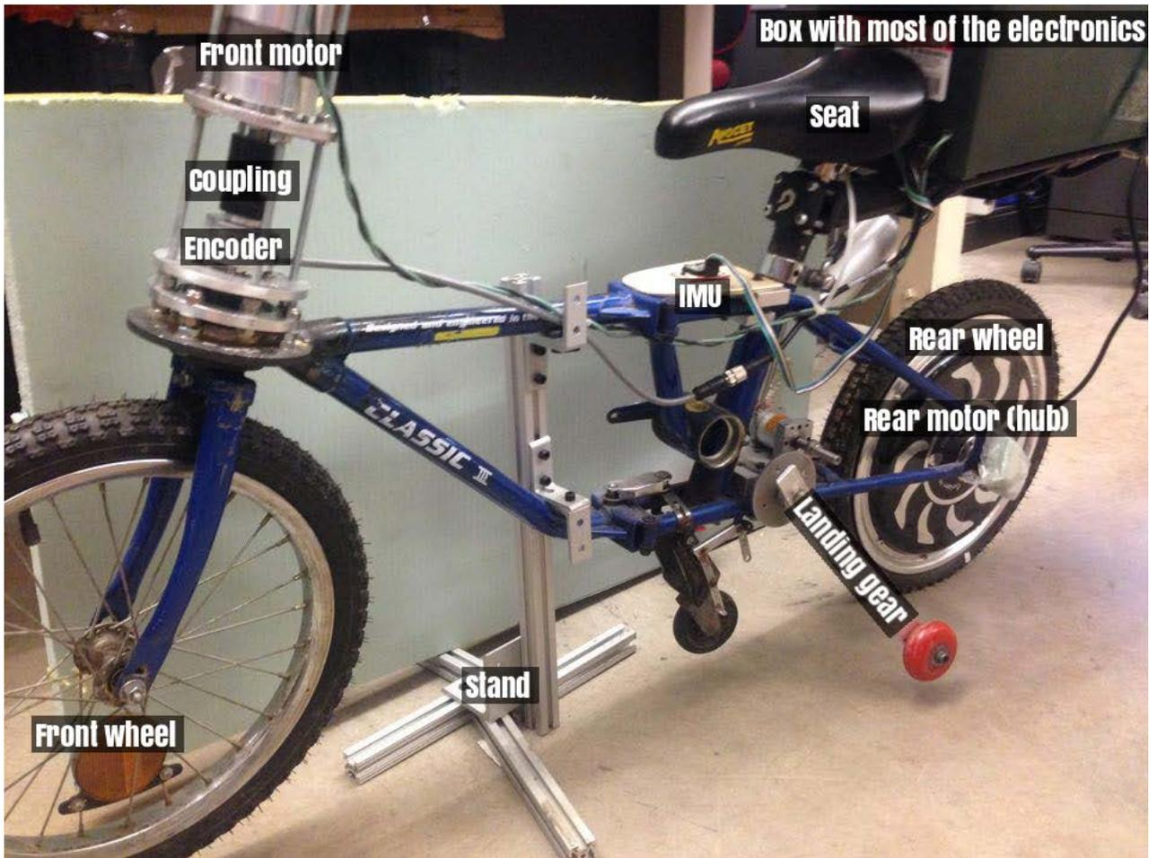
Figure 3.1: Complete bike diagram
