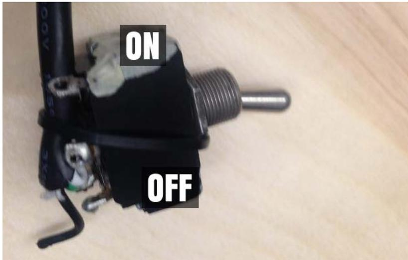
Figure 3.5: External switch for battery
