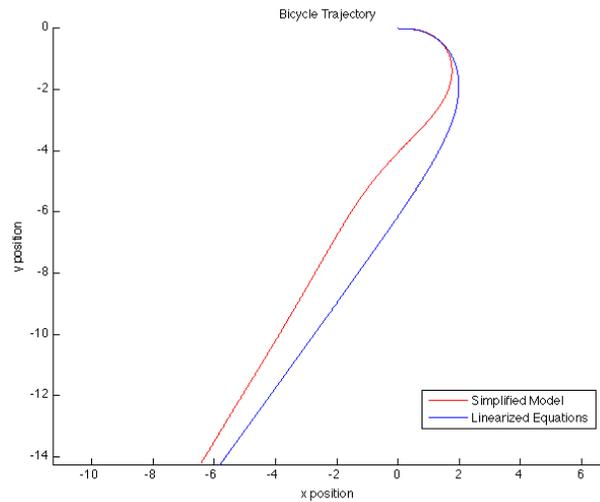
Figure 3: Comparison of the Linearized Equations and the Point Mass Bicycle Equations
