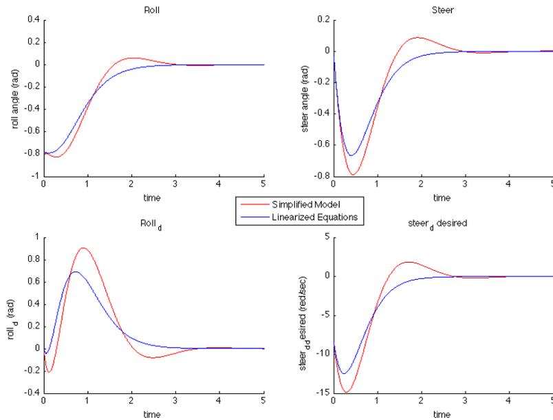
Figure 2: Comparison of the Linearized Equations and the Point Mass Bicycle Equations
