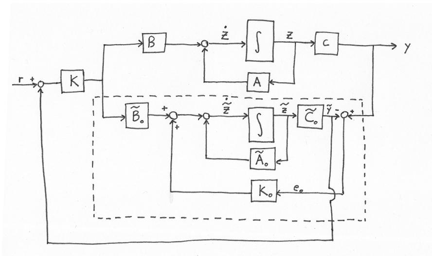
Figure 7: Observer Controller For Reference Tracking Block Diagram
