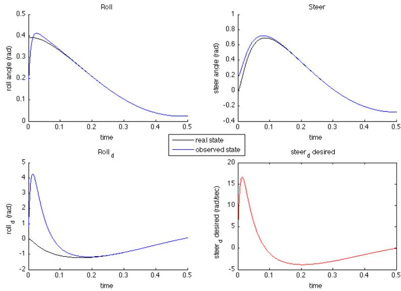
Figure 8: Observer Transient Behavior (on the Timescale of Milliseconds)
