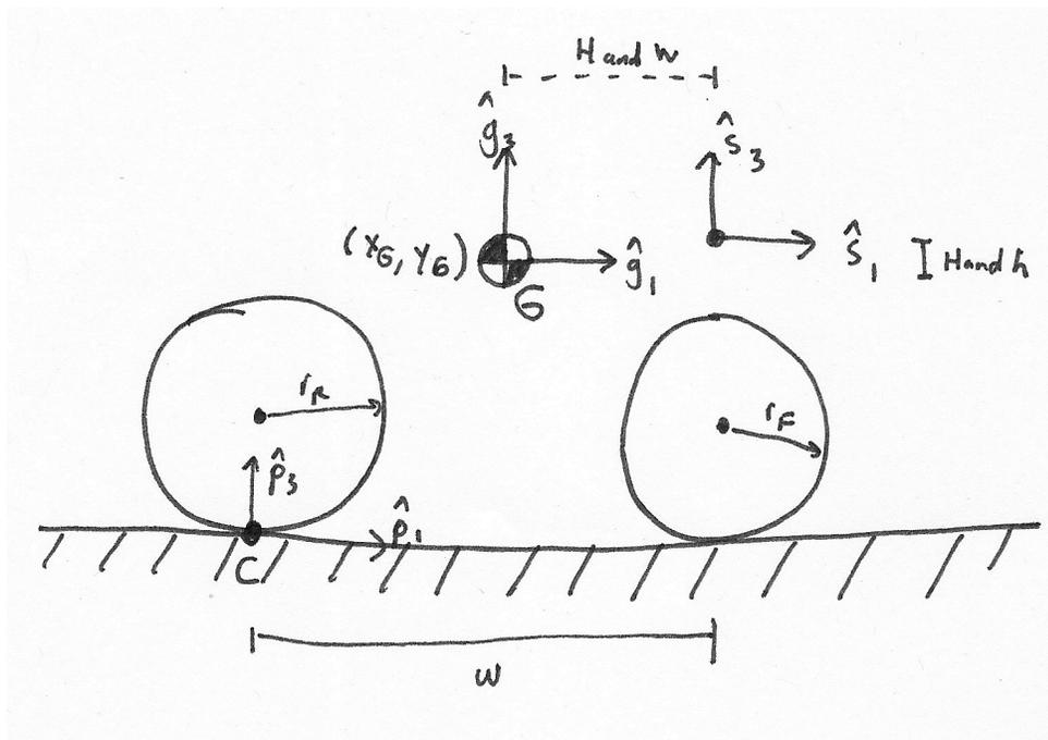
Figure 13: Bicycle Parameters and Frames
