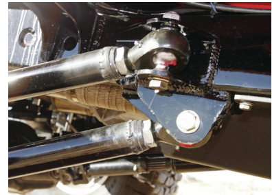
Figure 2.49: A rod end. Shown here in a jeep. A steel sphere slides in a truncated spherical cavity encased in the ‘rod end’. Often the cavity is brass encased in the steel rod end. In this case, a lubrication grease-fitting nipple is also visible. (From four-wheeler.com)
