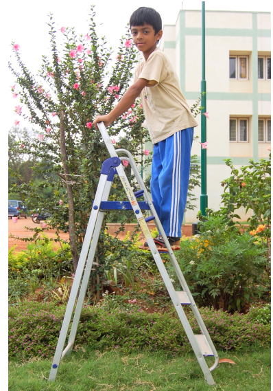
Figure 6.52: A ladder is well-modeled as a collection of rigid pieces connected by pin joints ...
