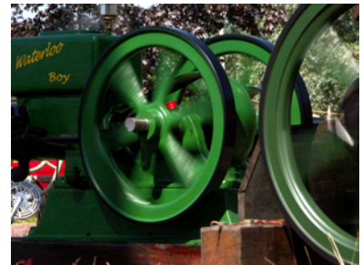
Figure 13.2: All points on a flywheel move in circles. The points further from the center move faster, so they move further while the camera shutter is open, so they show a bigger motion blur (the constant-thickness spokes look fatter near the rim).
