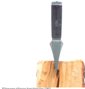
Figure 6.28: A hatchet splitting wood is a classic wedge. In this case it is used dynamically, with the force coming from the deceleration of mass. But other more complex wood splitting devices push the wedge in slowly.
