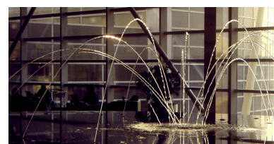
Figure 11.4: The water runs in continuous streams. Some fancy valve work (under the visible part of the fountain) is required to get such a laminar stream that holds together for the whole flight. This water draws its own graph of the trajectory of its particles. You can do the same kind of thing with a squirt gun next to a blackboard.
