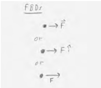
Figure 9.5: Two possible free body diagrams for 1D particle motion. It is assumed that \vec{F} represents the sum of all forces acting on the particle. Note, even though the inertial term m\vec{a} is of special interest, it does not show on the FBD. See the free body diagram Chapter 3 for the prescription about this. See box 9.2 on page 434 for a further warning about D'Alembert 'forces'.
