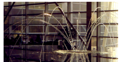
Figure 10.4: The water runs in continuous streams. Some fancy valve work (under the visible part of the fountain) is required to get such a laminar stream that holds together for the whole flight. This water draws its own graph of the trajectory of its particles. You can do the same kind of thing with a squirt gun next to a blackboard.
